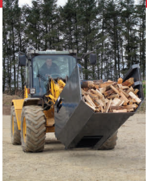
Ejector Bucket for filling Biomass Boiler
